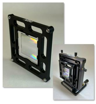
C2XXXS-BC 2-inch cylinder CGH mounted in C3 mechanical cell with 1/4" magnetic mounting balls (left). CGH mounted in FP3-Z-H425 6 degree of freedom alignment stage with linear Z -axis (right).
